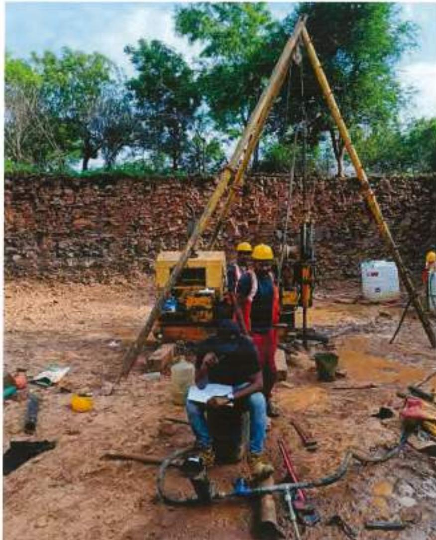
**Figure 5 : In-situ permeability Test in progress (SBH-01)**
