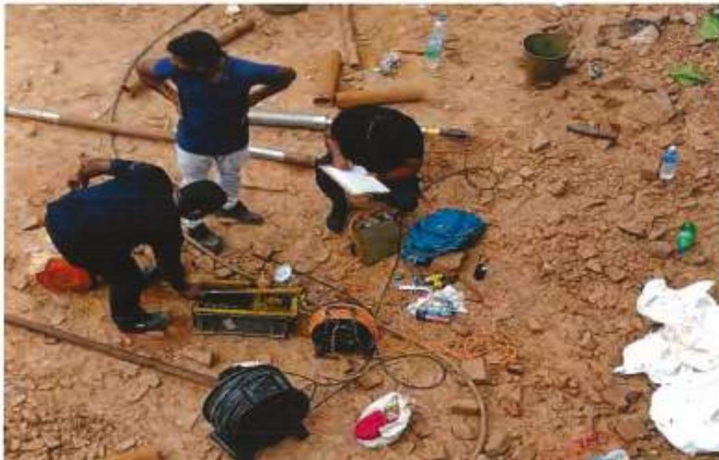
Figure 12 : Dilatometer test in Progress at Site
